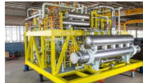
Gas de-hydration/dew point control
