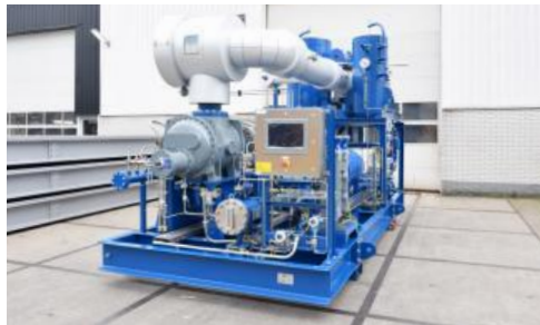
Vapor recovery unit
